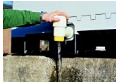
Arriving on site, insert the tap and distribute water. The tap in the picture has a simple flow control device designed for forming a narrow water jet.
