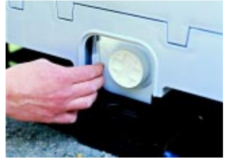
Snap gland adapter into place.
